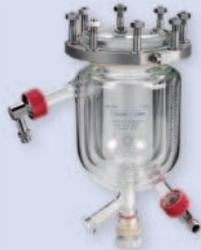
with bottom valve and tripple jacket for low temperature
